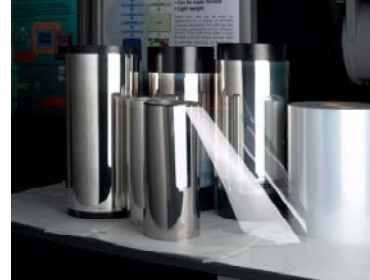
Flexible barrier substrates enable greater cost savings in manufacturing such as in allowing roll-to-roll processing.
